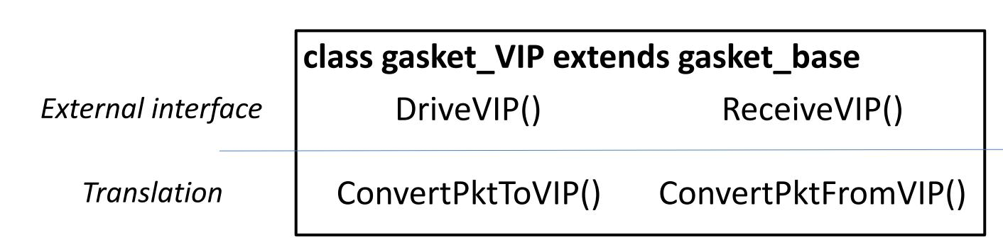
The VIP-specific gasket implements the pure virtual functions *only* to connect the VIP to the test bench. The DriveVIP/ReceiveVIP functions are a driver and monitor.
