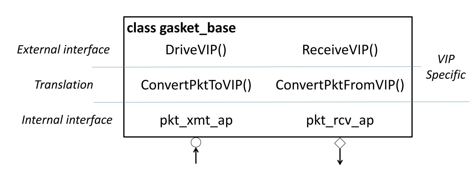
The base gasket fully defines the internal interface functions, while the VIP-specific portion is left pure virtual. The test bench at large accesses the VIP *only* through gasket interfaces.
